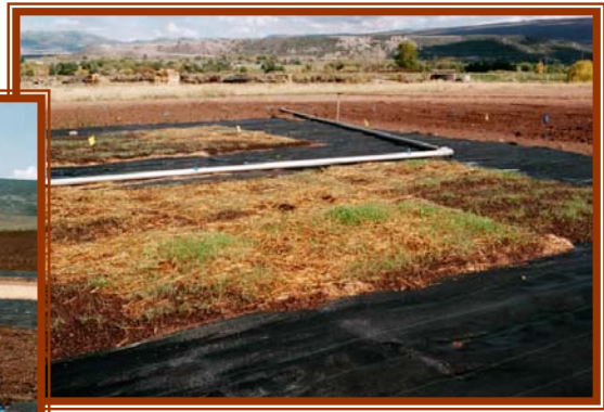
Plots with sprinkler irrigation as plants are emerging from mats. Weed barrier as base membrane in black.
