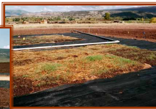
Plots with sprinkler irrigation as plants are emerging from mats. Weed barrier as base membrane in black.
