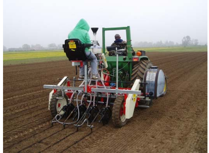
Use of a new 4-row Hege cone seeder for precision planting of grasses and forbs for seed increase. The PMC added the tank (far right) and spray nozzles to apply activated carbon bands over each seeded row. A nonselective herbicide is sprayed shortly afterwards for weed control between rows. The carbon protects the crop seed.
