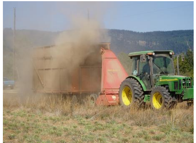
Hiniker Flail Mower/Shredder similar to the one purchased by the PMC. The wagon collects the material.
