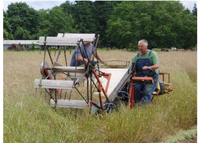
The "moon rover" is used to harvest mature seed heads (in this case those of California brome) or flower stalks directly in the field. The material is cut then bagged off the conveyor belt, and later dried and mechanically threshed in a separate operation. The machine is named after the designers/builders Carroll Moon and Daryl Ehrensing of Oregon State University.
