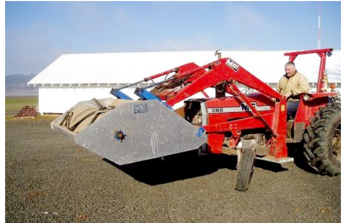
This flail-vac seed stripper uses a high speed brush to strip seed off the heads of grasses and dry flower stalks of forbs. It is controlled like the bucket on a front end loader. The unit has proven to be effective for harvesting several species.
