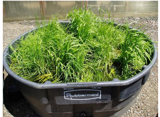
Cattle trough used to evaluate water depth tolerance of several grasses grown in pots and anchored at different elevations.
