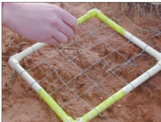
Figure 6.1 Quadrat frame used for point-cover estimation. This frame is 25 x 25 cm in size. Hits are determined by dropping a pin vertically from each intercept within the frame.
