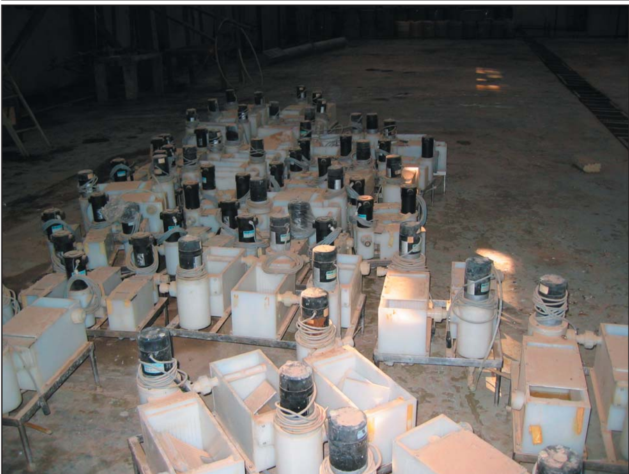
Figure 26. Mixer-settlers in storage at Ibn Sina (photo taken by ISG Team, December 2003).
