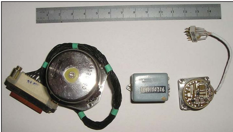
Figure 28. MG-4 gyroscope, AK-5 and A-15 accelerometers.
