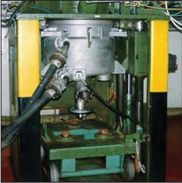
Figure 8. 30-gallon/100-liter propellant mixer bowl.
