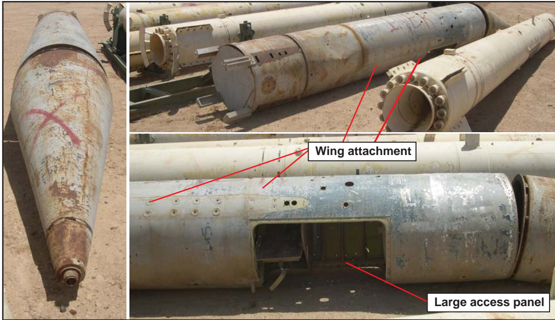
Figure 3. Early Al Samud II using HY-2 airframes.
