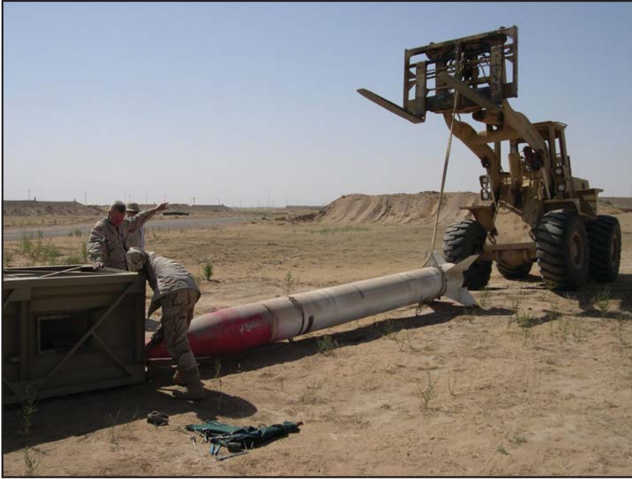
Figure 17. Al Fat'h missile with submunition warhead.
