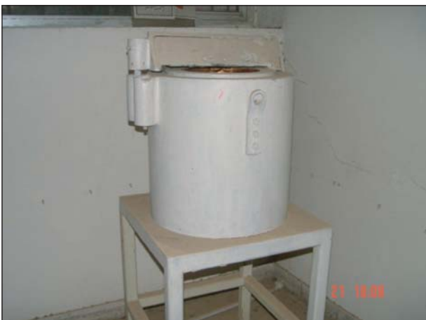
Building 59: Rad. source-led cave (R45).
