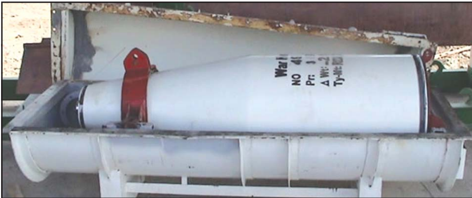
Figure 9. Al Fat'h unitary warhead in a shipping container.
