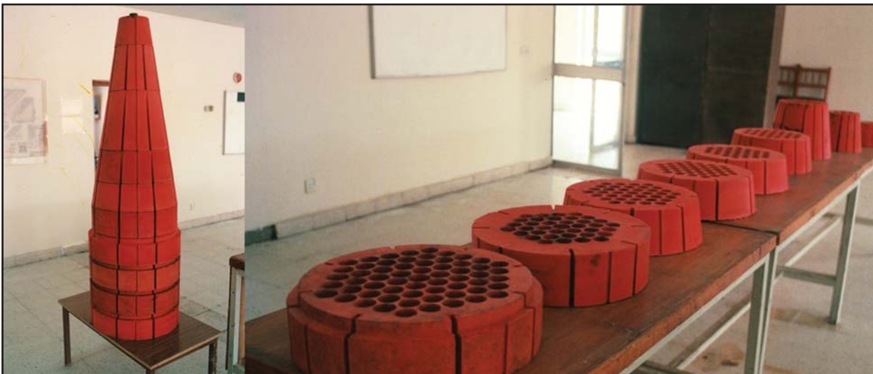
Figure 12. Lightweight foam moldings used in the Al Fat'h warhead.
