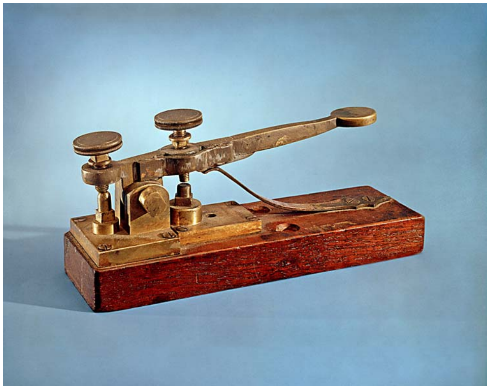
Morse/Vail telegraph key, 1844. The telegraph key Samuel Morse used on his first line in 1844 was very simple--a strip of spring steel that could be pressed against a metal contact. This telegraph key is part of the collection of the National Museum of American History, which is closed for renovations until the summer of 2008. Smithsonian Photo by Alfred Harrell.
