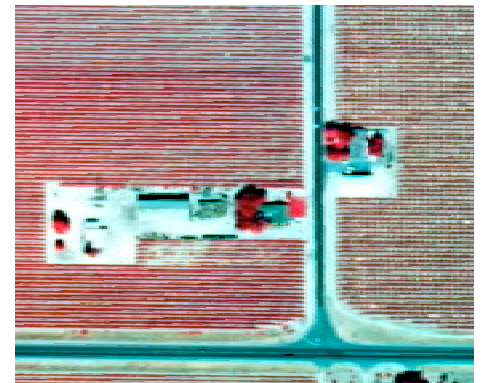
False Color Infrared: Digital image with the near infrared band substituted for the green band. The near infrared band indicates plant stress and level of vigor.
