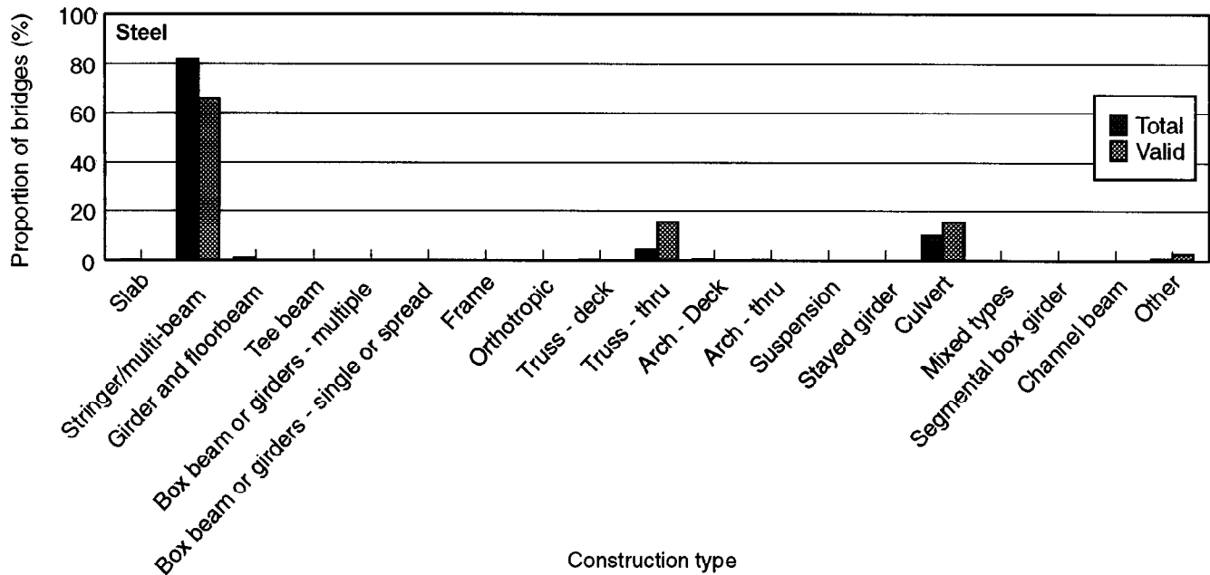
Figure 37—Percentage of steel bridges from the valid set and total population by construction type.
