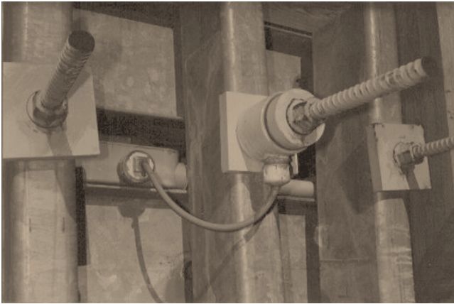
Figure 15—One of six load cells installed on stressing bars to monitor changes in bar tension.
