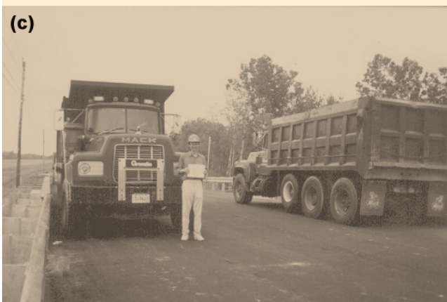
Figure 18—Truck positions for load test 1 for three load cases (looking north): (a) load case 2, (b) load case 3, (c) load case 6.
