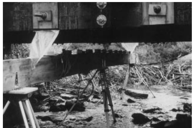
Figure 16—Load test 2 bridge deflections were measured with string potentiometers attached to the underside of the bridge. The transducers were supported by a wood beam and tripods.
