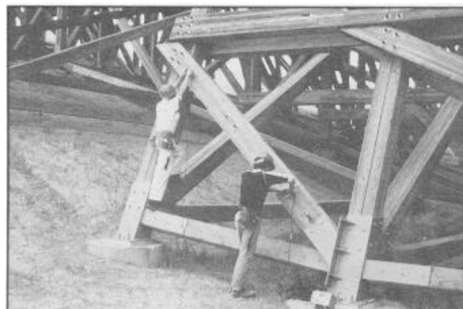
Figure 21—Stress wave evaluation of wood members of TRESTLE.
