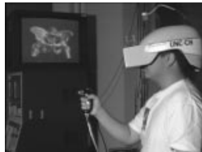
Figure 8. - David Chen pictured using a head mounted display. Stereo surface renderings are presented in a virtual environment for medical visualization.
