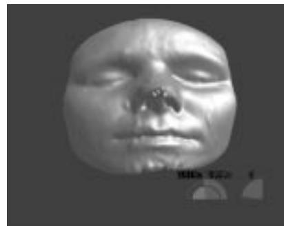
Figure 7. - MR head study (96x96x109 voxels). Skin surface (269720 triangles) generated in 591 msec. Update rate 3 fps
