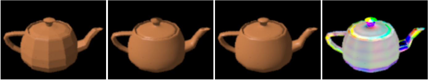
Figure 3. Comparison of linear normal interpolation with parametric normal interpolation. Left: 504 polygonal facets. Middle left: Shading with linear normal interpolation. Middle right: Parametric normal interpolation. Right: Difference of normals for middle images.
