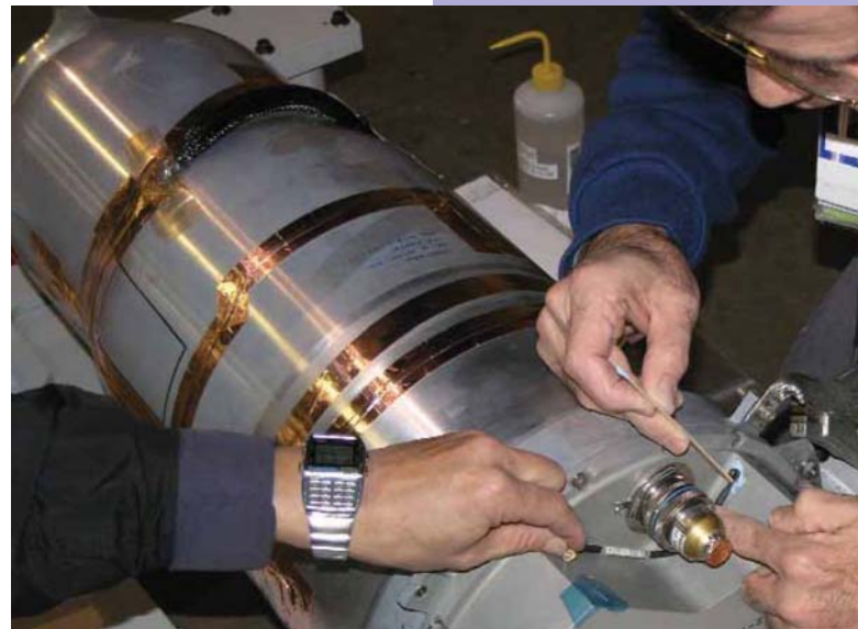
Technicians attach instrumentation to the exterior of a W80 Environmental Test Unit.
