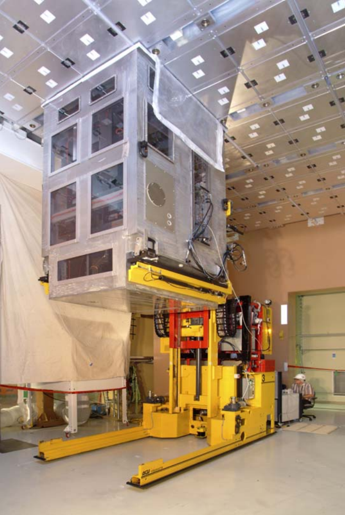
The 1000th line-replaceable optical unit is maneuvered into position at the National Ignition Facility at Lawrence Livermore National Laboratory.
