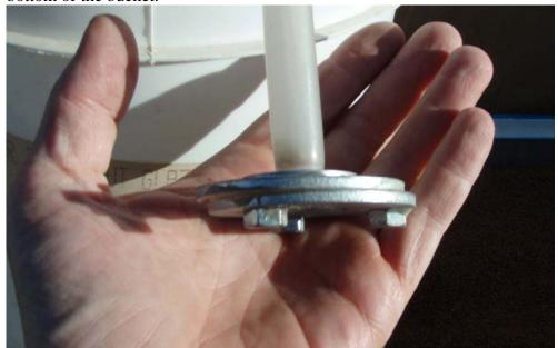
The intake end of the tube has been heated and fared to secure it into the weight
