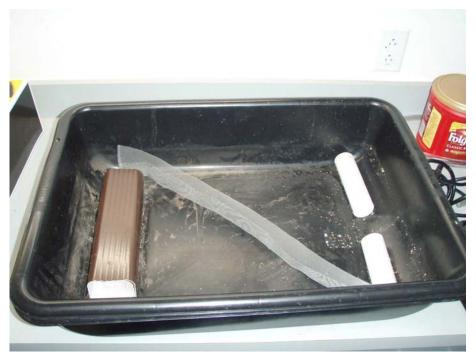
The upper support is made out of a section of down spout, the bottom two short lengths of PVC pipe with an opening between them for the drain hole from the top pan. The holder for the hose on the top pan is made out of a section of tubing with its ends cut at an angle and a fair amount of hot melt glue.
