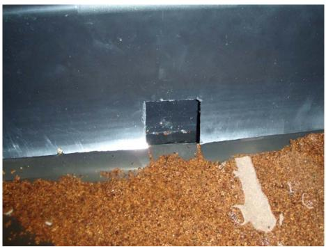
When running, stream channel features will form. The bottom opening can be dropped to create features such as head cuts and scour holes.
