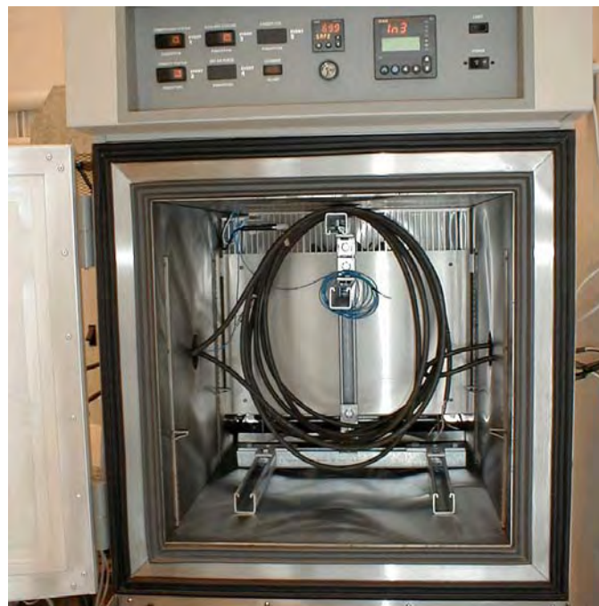
Figure 15 Typical aging chamber loading for global and hot-spot aging of cable test specimens
