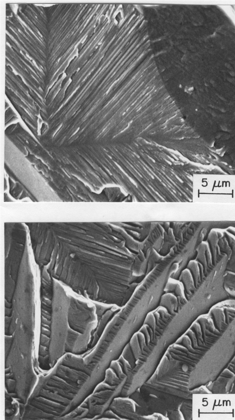
Figure 33. Herringbone Cleavage in Heat P4 Aged for 10,000 h at 400°C and Tested at Room Temperature.
