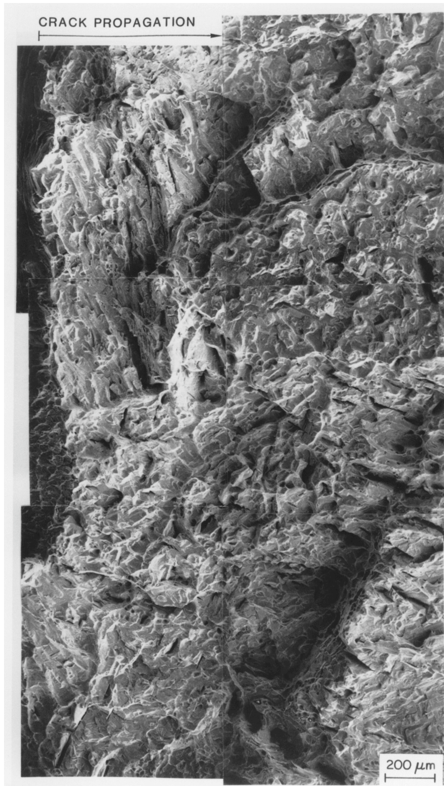
Figure 27. Fracture Surfaces of Aged CF-8 Cast Steel Tested at Room Temperature. (a) Heat 68, 21% ferrite and (b) Heat 60, 21% ferrite. Crack propagation from left to right.
