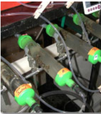
Examples of the acrylic minipipes used in the tests. The pipe with clear water on left is an untreated control, whereas water in other pipes has a grayish color due to presence of suspended bacteria during treatment. Mussels are visible attached to walls of pipe.
