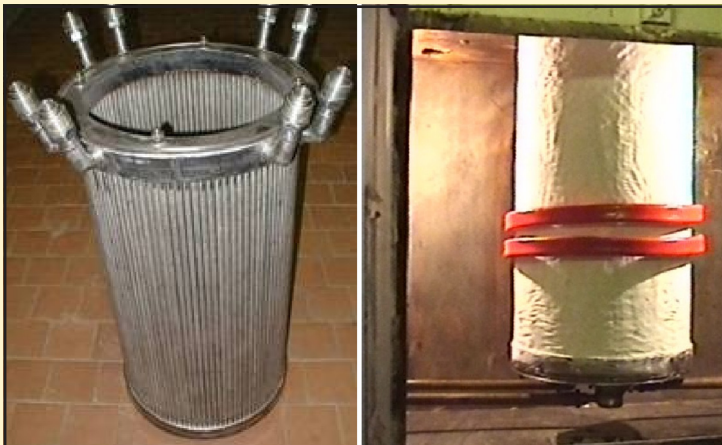
From Left to Right: 1) Cold Crucible Melter at SIA Radon before insulation and 2) After insulation with induction heating coils.
