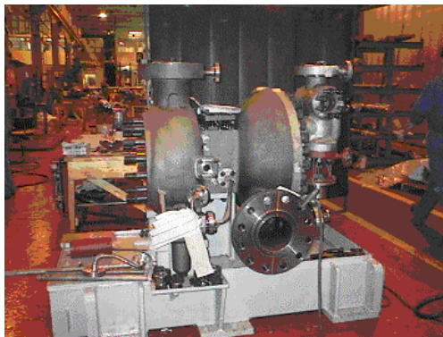
Figure 3.5-7 The RCIC Turbine-pump for Lungmen
