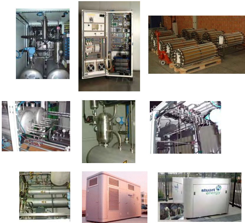
Figure 3B-9. Components from Stuart Energy Systems Electrolyzer
