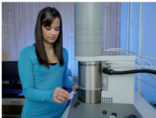
Marisa Arnold holding a sample for the Laser Flash Apparatus.
