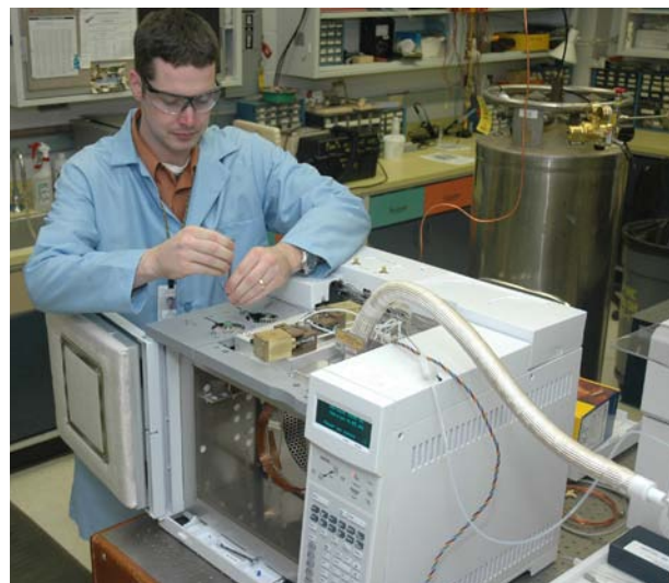
NETL researcher Kirk Gerdes injects a sample into NETL's new gas chromatograph-inductively coupled plasma-mass spectrometer, an analytical instrument that will play an important role in studying the effect of coal contaminants on solid oxide fuel cells.
