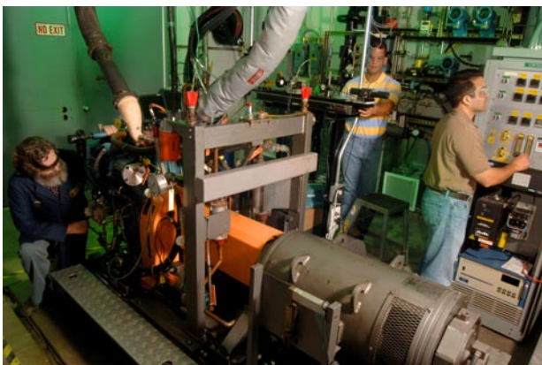
Researchers prepare NETL's Ricardo Proteus engine for hydrogen-fueled test operation.
