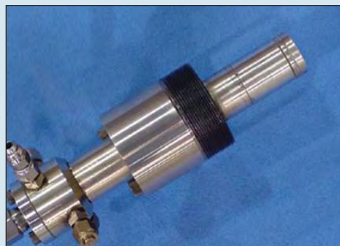
CCADS sensor inserted into the center body of a fuel nozzle
