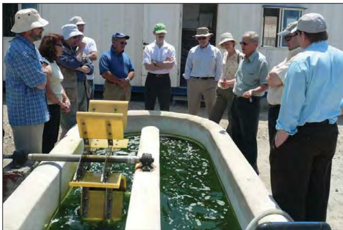
The algae tank at the Ashkelon coal-fired power plant cultivates algae for pills, a diet supplement common in Japan. A similar process could be used for sequestration, and is being developed by Arizona Public Service for its Redhawk Plant
