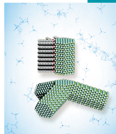
CdTe nanotetrapod. The growth rates of two crystalline phases of CdTe are balanced to grow tetrapods for use in advanced solar cells.
