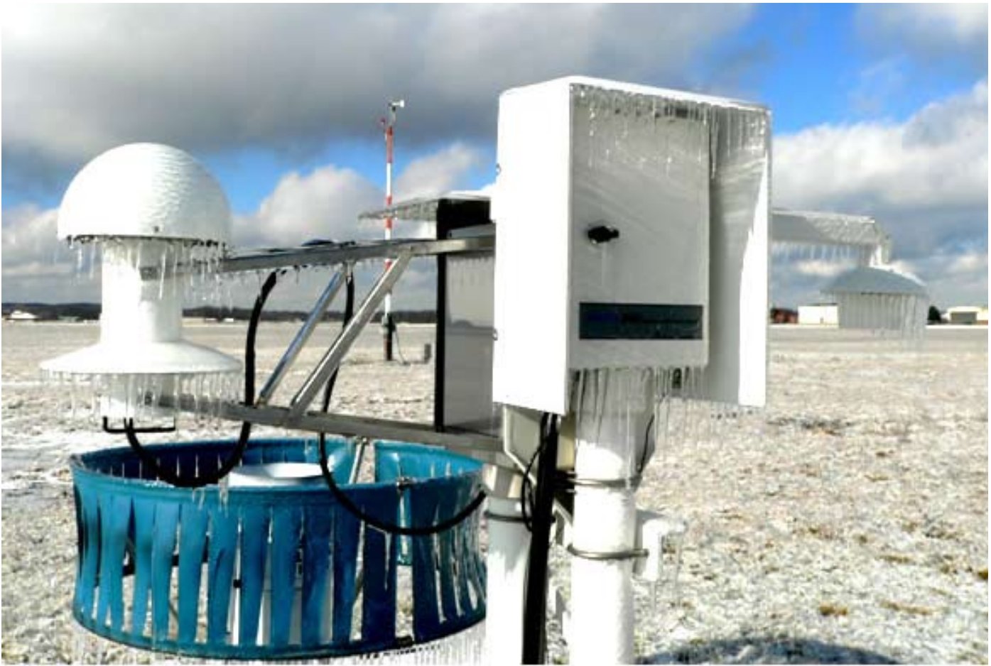
Shown above are a frozen temperature sensor, dewpoint sensor and heated tipping bucket on an ASOS unit. In the past, during periods of icing or freezing precipitation an entire array of ASOS weather equipment could freeze up or malfunction. ASOS now includes an Ice Free Wind Sensor as well as improved freezing rain sensors. Photo by NWS Grand Rapids, MI, Electronics Technicians Eric Repaal and Thomas Williams.
