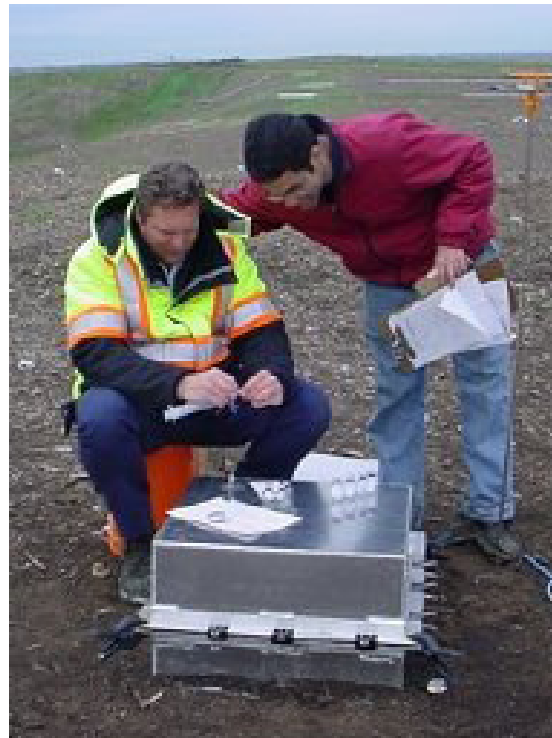
Figure 3 – Apparatus for measuring solid waste properties at the Yolo County facility
