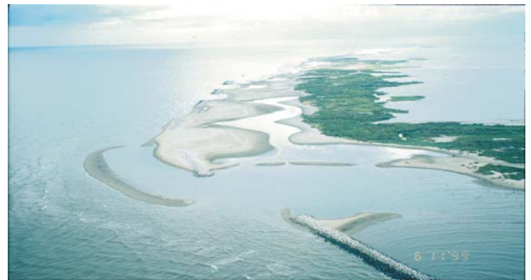
Sand deposits or "tombolos" have developed behind the breakwaters that protect and enhance the island. A similar effect is expected to occur behind the 8 additional breakwaters being constructed to the west of the existing project.
