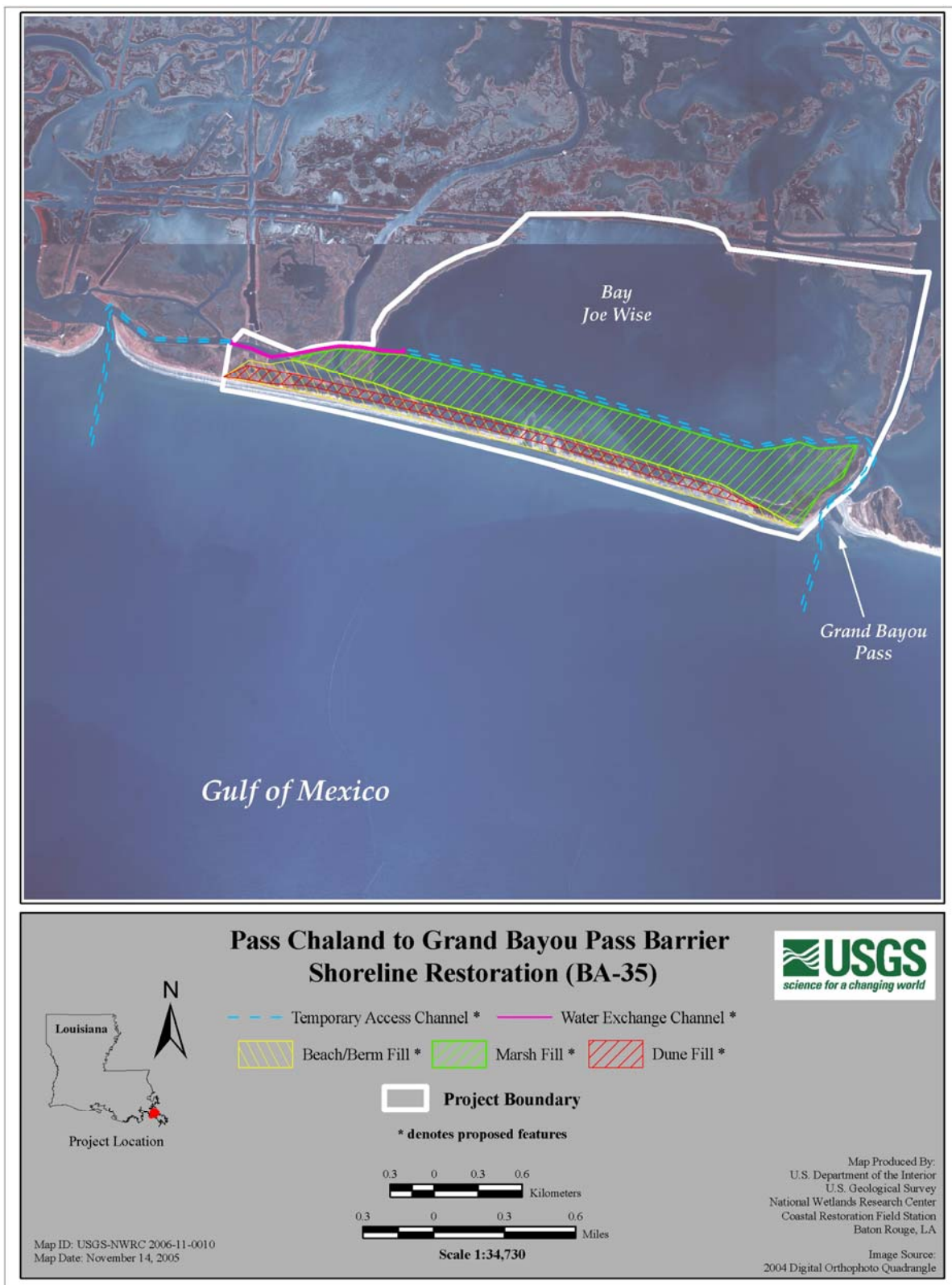
Figure 2: Phase II Project Feature and Boundary Map
