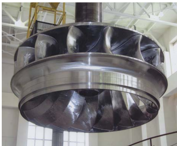
Turbine runner replacement at Shasta Powerplant
