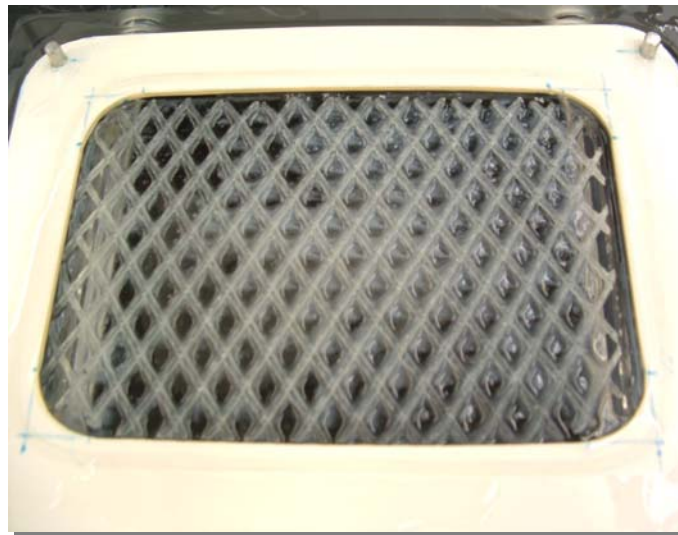
Figure 15. Photograph showing the scale on the spacer used during Brine B VEDCMD experiments.
