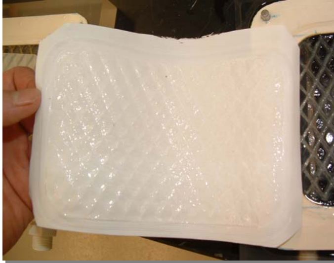
Figure 14. Photograph of the scale formed on the membrane during the Brine B VEDCMD experiments.
