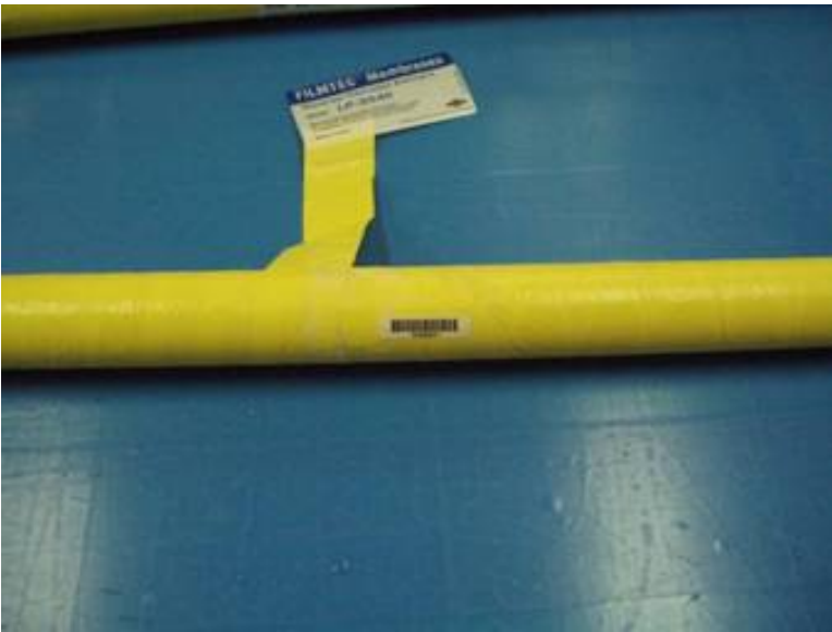
Photo 5: tape and label came loose
