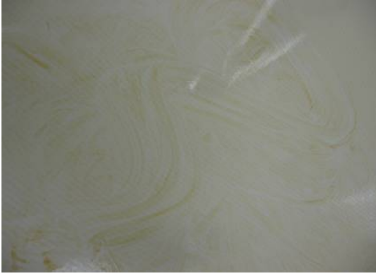
Photo 6: rusted color foulant covers on membrane surface
