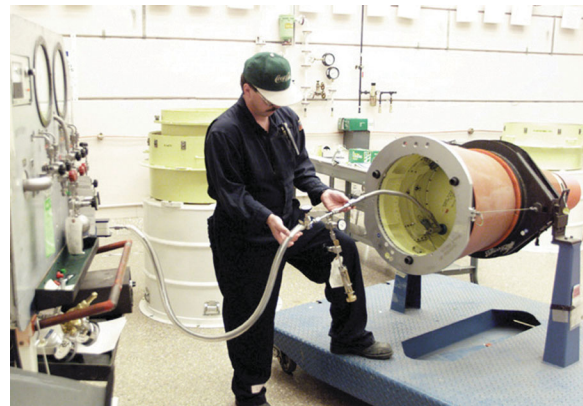
A technician uses a solid-phase microextractor to collect samples of gases produced by organic materials in a weapon.
