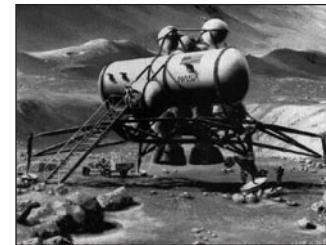
Mars Excursion Vehicle would have transported four astronauts and 25-tons of cargo to Martian surface (Source: 90 Day Study)
