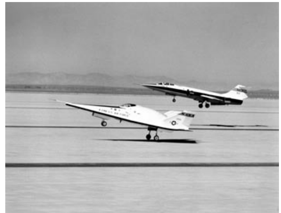
Landing a lifting body. The wingless X-24B required a particularly high angle of attack. (NASA)
