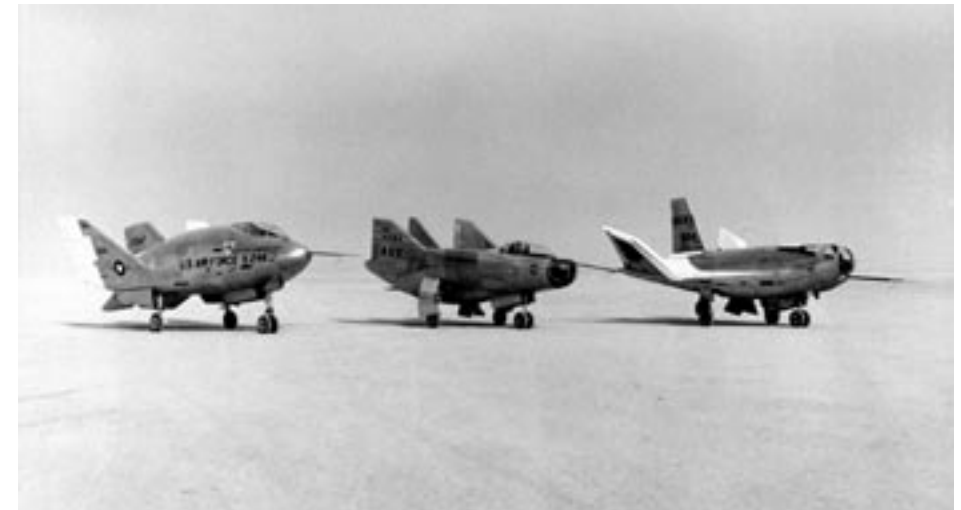
Lifting bodies. Left to right: the X-24A, the M2-F3 which was modified from the M2-F2, and the HL-10. (NASA)
