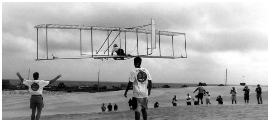
Lieutenant Commander Klaus Obman, U.S. Navy, pilots the 1902 replica on 6 October 2002. At an altitude of 12 to 15 feet, the glider will stay in the air 12 to 15 seconds, traveling 125 to 150 feet down the slope of the dune on this flight. (Photograph by Scott Carpenter, courtesy of the Western Reserve Historical Society)
