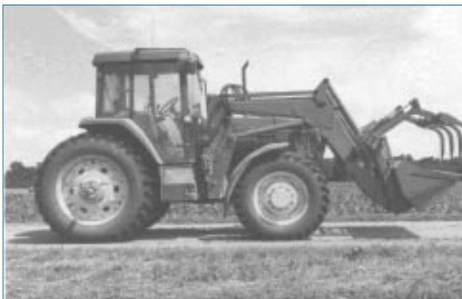
Photo 1. The tractor shown above has a front-end loader equipped with an attachment for securing bales (grapple). The loader is shown in a lowered position, which is the safest position to use when moving bales.
