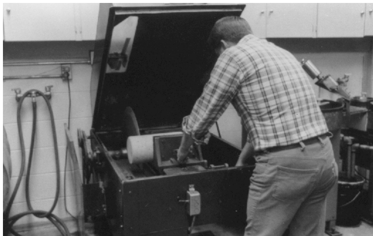
Figure 4. Large, oil-cooled, continuous diamond-edged rotary saw.
