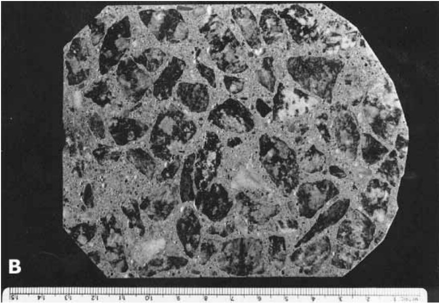
Figure 63. Finely lapped slices of concrete with abnormal paste content (actual size): High paste content.
