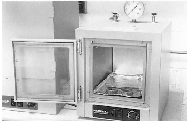
Figure 16. Vacuum oven: Thin-section stock in liquid dyed epoxy in small disposable dishes.
