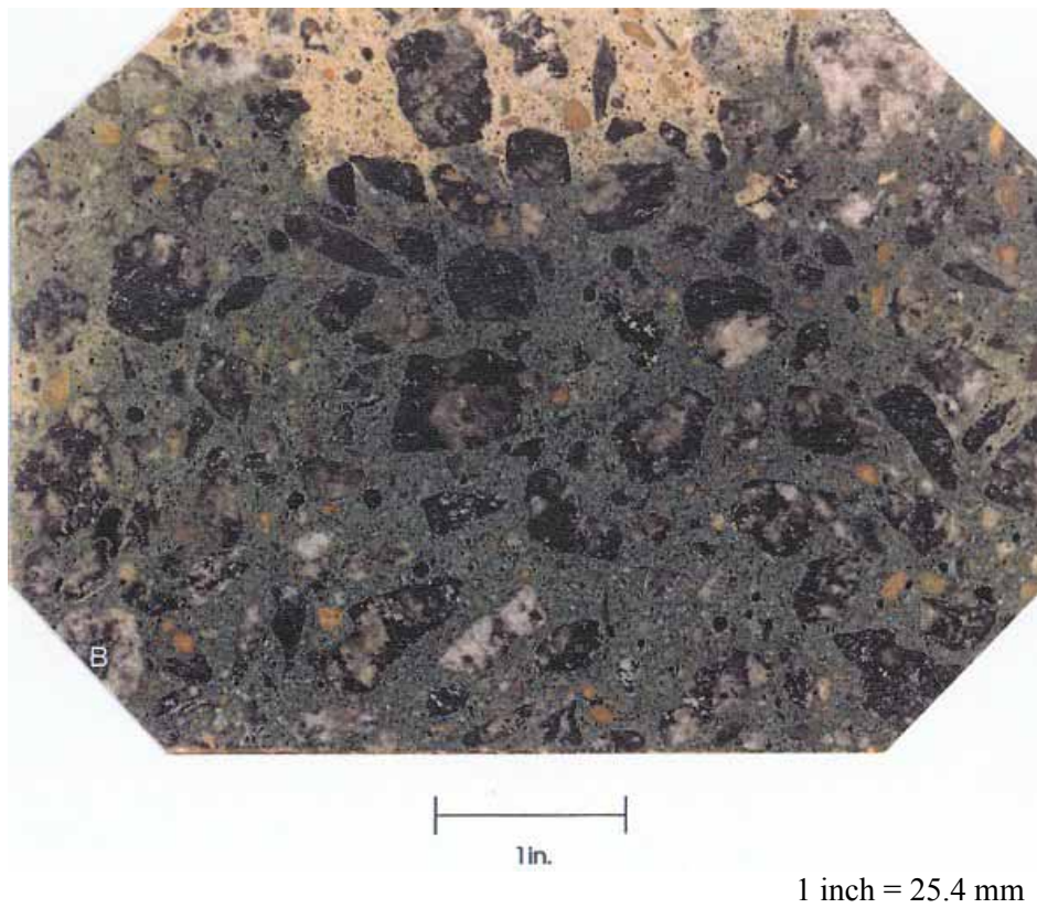
Figure 140. Interior of beam of HCC containing slag, illustrating the partially dry two-color stage.
