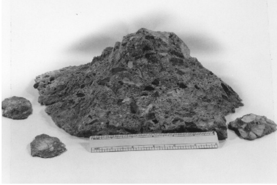
Figure 203. Giant popout caused by a piece of glass (accompanying it are several small popouts of a more usual size caused by porous chert particles).
