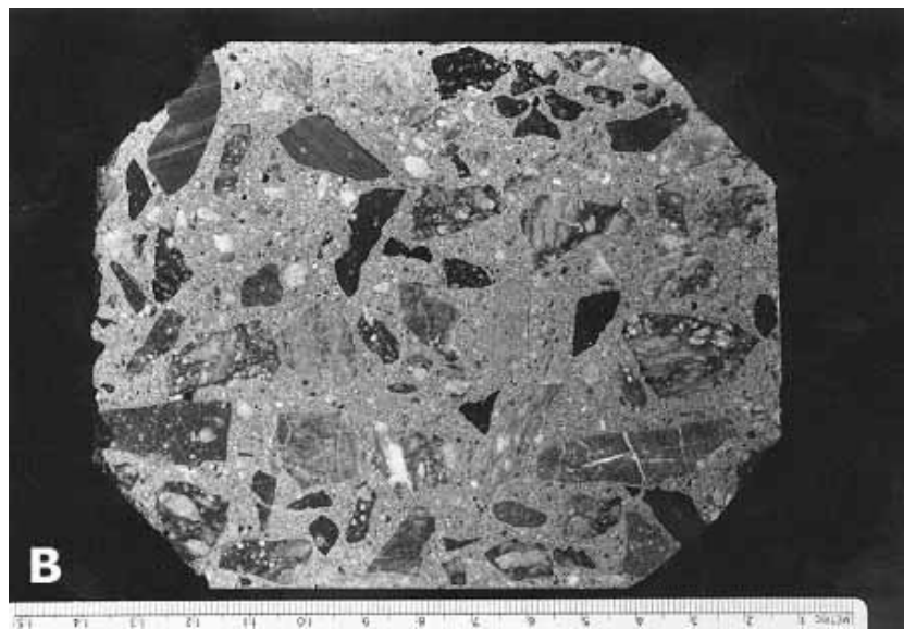
Figure 62. Finely lapped slices of concrete with normal paste content (actual size): Angular crushed granite coarse aggregate and fine sand aggregate.
