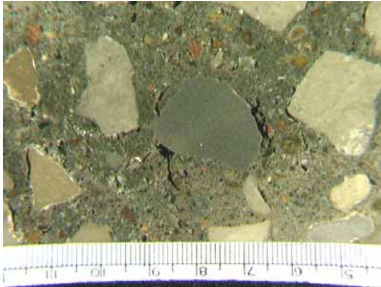
Figure 67. Knot of cement exposed on finely lapped slice (rounded shape was caused by tumbling in the mixer).
