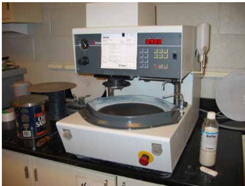
Figure 10. Automated grinding, lapping, and polishing machine uses interchangeable grinding and polishing discs to simplify specimen preparation.
