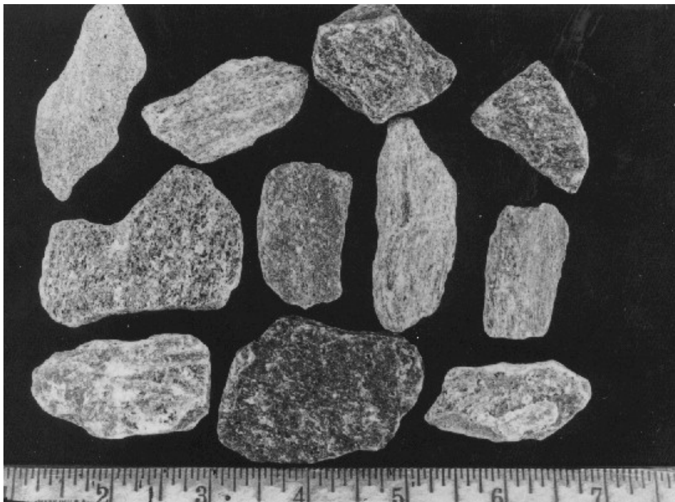
Figure 207. Aggregate particles from a fissile gneiss (a particle shape such as this can cause a high water demand).
