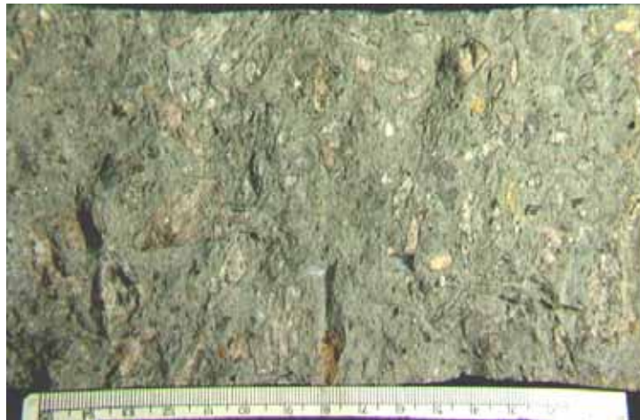
Figure 105. Fracture face of splitting tensile specimen: Examine for aggregate fracture and deterioration, as well as secondary deposits.
