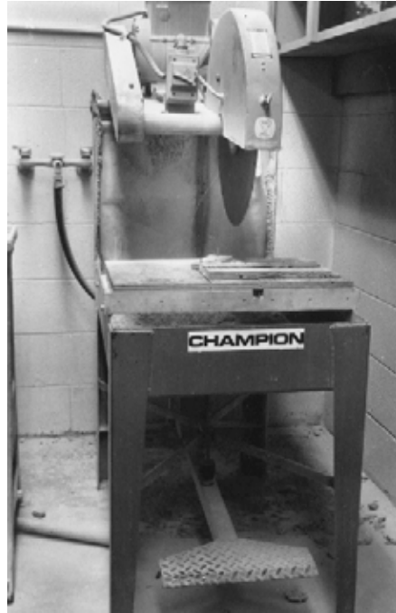
Figure 3. Water-cooled, segmented, diamond-edged rotary saw with overhead arm (360-mm blade is diamond-edged and slotted into wide teeth; foot pedal controls the height of the saw).
