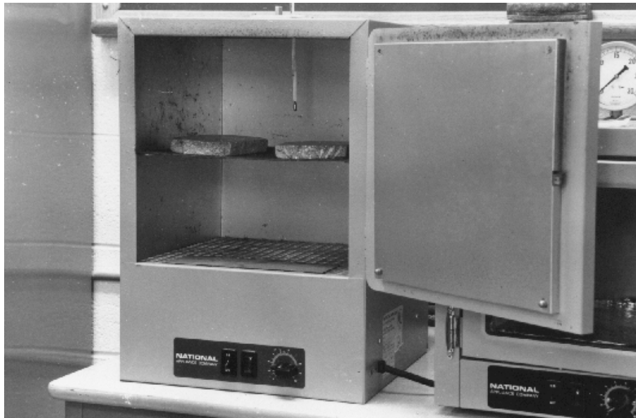
Figure 15. Drying oven (thermostatically controlled).
