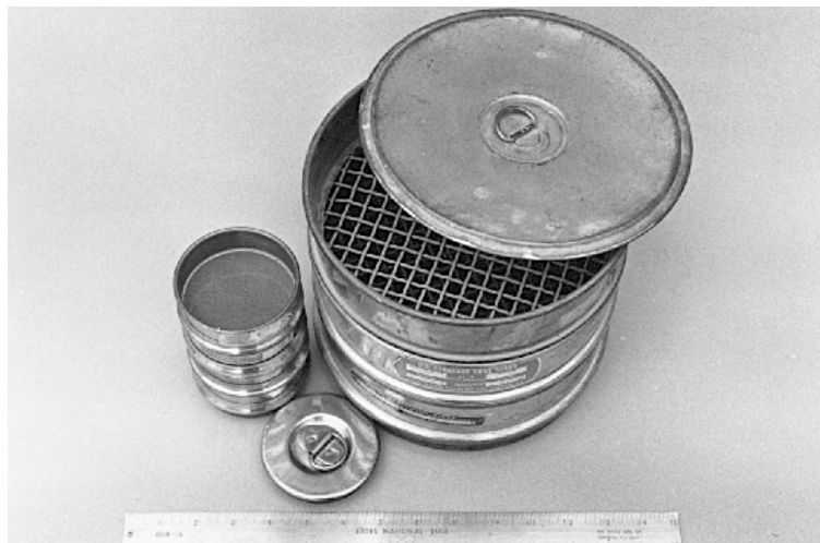
Figure 22. Types of sieves used in examination of concrete and concrete materials (203-mm and 76-mm sizes).
