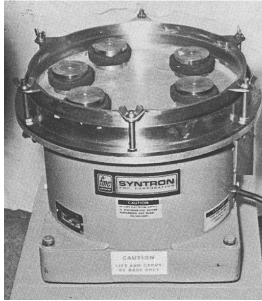
Figure 19. Syntron vibratory polisher and weights (weights have sponge rubber bumpers) (Walker and Marshall, 1979).
