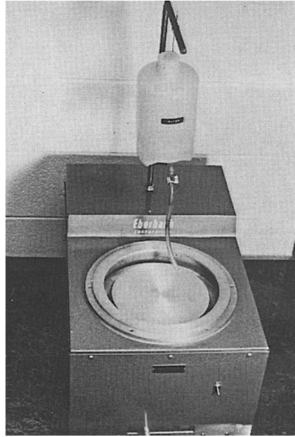
Figure 7. Bench lap (diameter of 200 mm, for rough-grinding rock and concrete specimens; suspended bottle is for water or another lubricant; grinding compounds may be shaken like salt from plastic bottles with a pierced cover).
