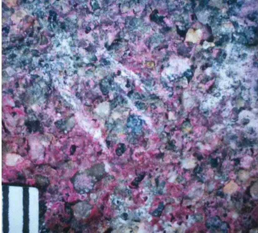
Figure 92. Fractured surface treated with \text{BaCl-KMnO}_4 (secondary deposits containing sulfate are stained pink).
