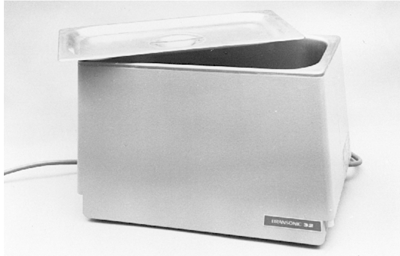
Figure 11. Ultrasonic cleaner (tank is of a material that will resist most solvents).
