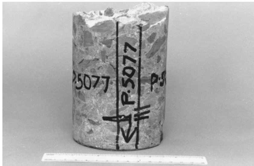
Figure 32. Core marked with identification, cutting planes, and match marks.
