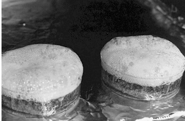
Figure 17. Closeup of bubbling of liquid epoxy as vacuum removes air and water from specimen.
