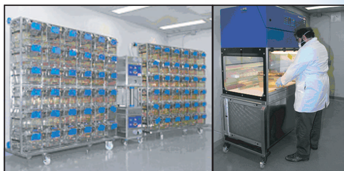
Containment caging and changing system
