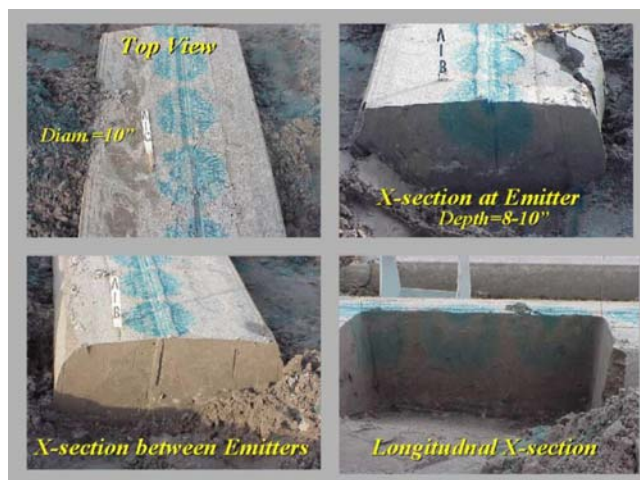
Figure 21. Top, side, and cross sectional view of a raised plant bed illustrating the small, circular wetted areas beneath individual drip irrigation emitters using a blue tracer dye injected into the irrigation water. Drip injection time of 2 hours.
