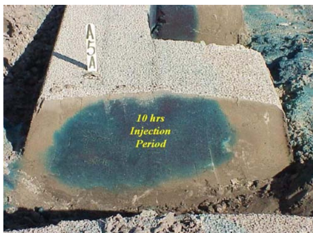
Figure 23. Cross sectional view of a raised plant bed illustrating how irrigation water may not move radially outwards to the sidewalls or shoulders of the bed, even after long irrigation cycles. A blue, water soluble, tracer dye is injected into the irrigation water to characterize drip water movement over time.
