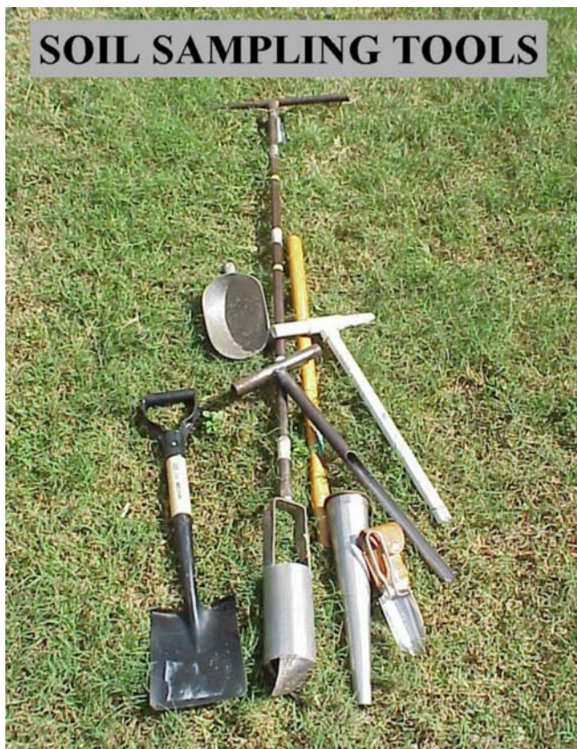
Figure 9. The collection of soil samples for nematode analysis can be acquired from the field using a cylindrical sampling tubes, trowels, or shovels.
