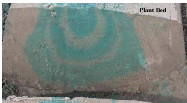
Figure 20. Illustration of the incremental radial expansion of the wetted zone in a raised plant bed after pulsing the injection of a blue, water soluble, dye applied through a drip irrigation system. Each ring represents 2 hours irrigation run and injection time.
