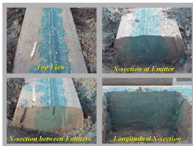
Figure 22. Top, side, and cross sectional view of a raised plant bed illustrating the development of a wetted strip after water fronts from adjacent emitters collide. A blue, water soluble, tracer dye is injected into the irrigation water to characterize drip water movement over time.
