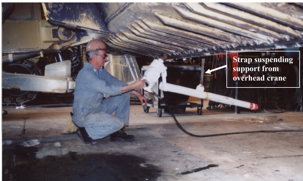
Figure 8.—Mechanic using a support to hold an impact wrench when changing the cutting edges on a dozer blade. The support is attached with a strap to an overhead crane.
