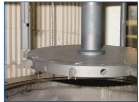
The Hostile Atmosphere Elevated Temperature Erosion test is used to study erosion and corrosion in a gas environment.
