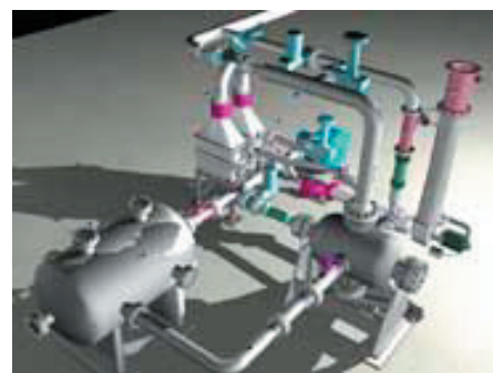
The Hyper facility allows assessment of dynamic control and performance issues in fuel cell-turbine hybrid systems.
