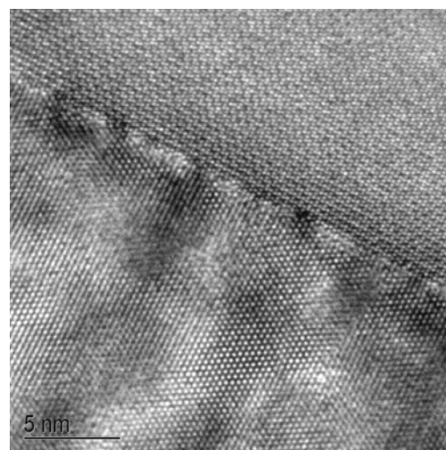
Figure 1. High-resolution transmission electron microscopy image showing the interface between \alpha -Al 2 O 3 and ZnO with the film grown on r-cut \alpha -Al 2 O 3 .
