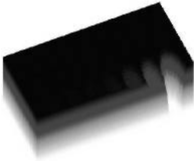
Figure 6. Three-Dimensional Detector Image. Three-dimensional rendition of the image of the "detector" end of the probe when the "target" end is in contact with and illuminates a subject's forearm with 543 nm light.
