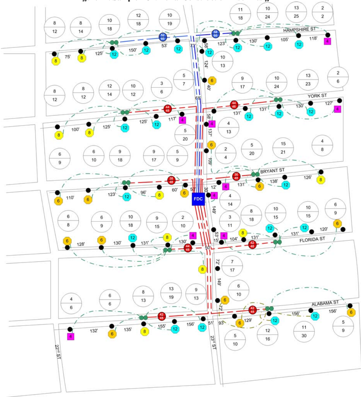
Figure 22: Sample PON Aerial Construction Fiber Design
