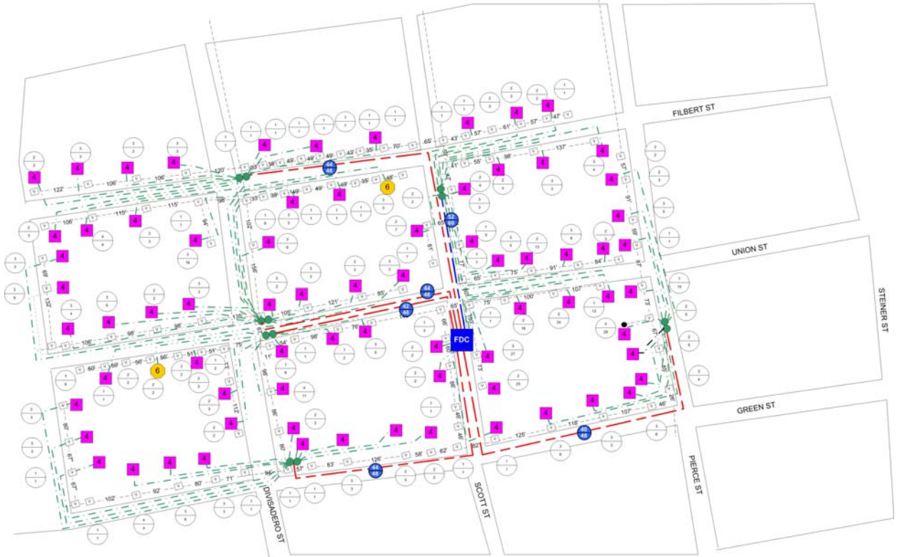
Figure 23: Sample PON Underground Construction Fiber Design
