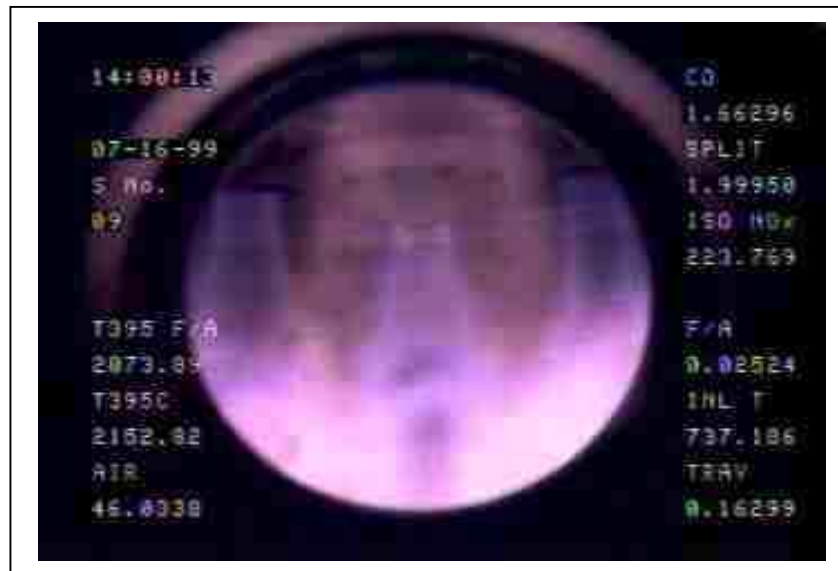
Figure 15: Video Capture of Flame Structure, 85-90% Hydrogen
